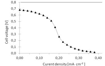
Fig. 3. Polarization curves of electrooxidation (with carbon electrode) of glucose from wastewater with bacteria from activated sludge
