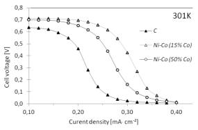
Fig. 8. Polarization curves of electrooxidation of wastewater with bacteria from activated sludge with carbon and Ni-Co alloy catalyst at the temperature of 301K
