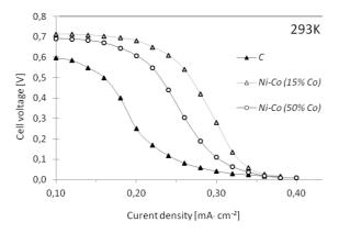
Fig. 4. Polarization curves of electrooxidation of wastewater with bacteria from activated sludge with carbon and Ni-Co alloy catalyst at the temperature of 293K
