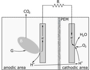
Fig. 1. Operating principles of a MFC. Figure is not to scale. PEM - proton exchange membrane, B - bacterium, G - glucose
